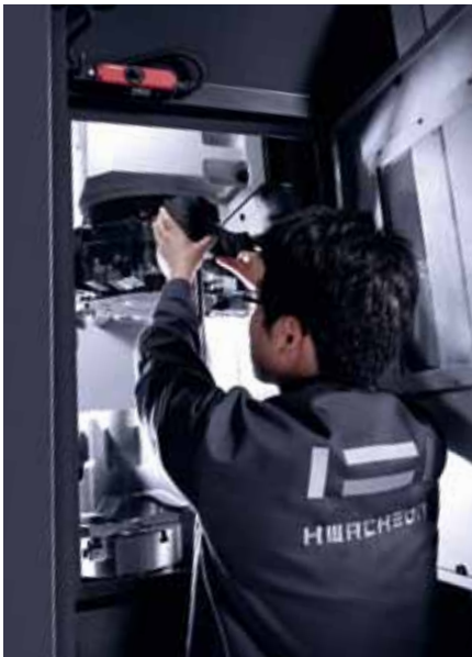
Changing tools is convenient when the ATC returns to its parking position, according to the side access door (VT-650)
