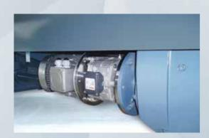
DURMA magnet brakes and clutch system is for
