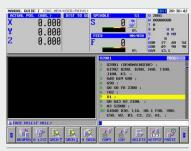
It displays the machine status and the tools in use while machining.
