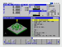
The realistic machining simulation checks the program.
